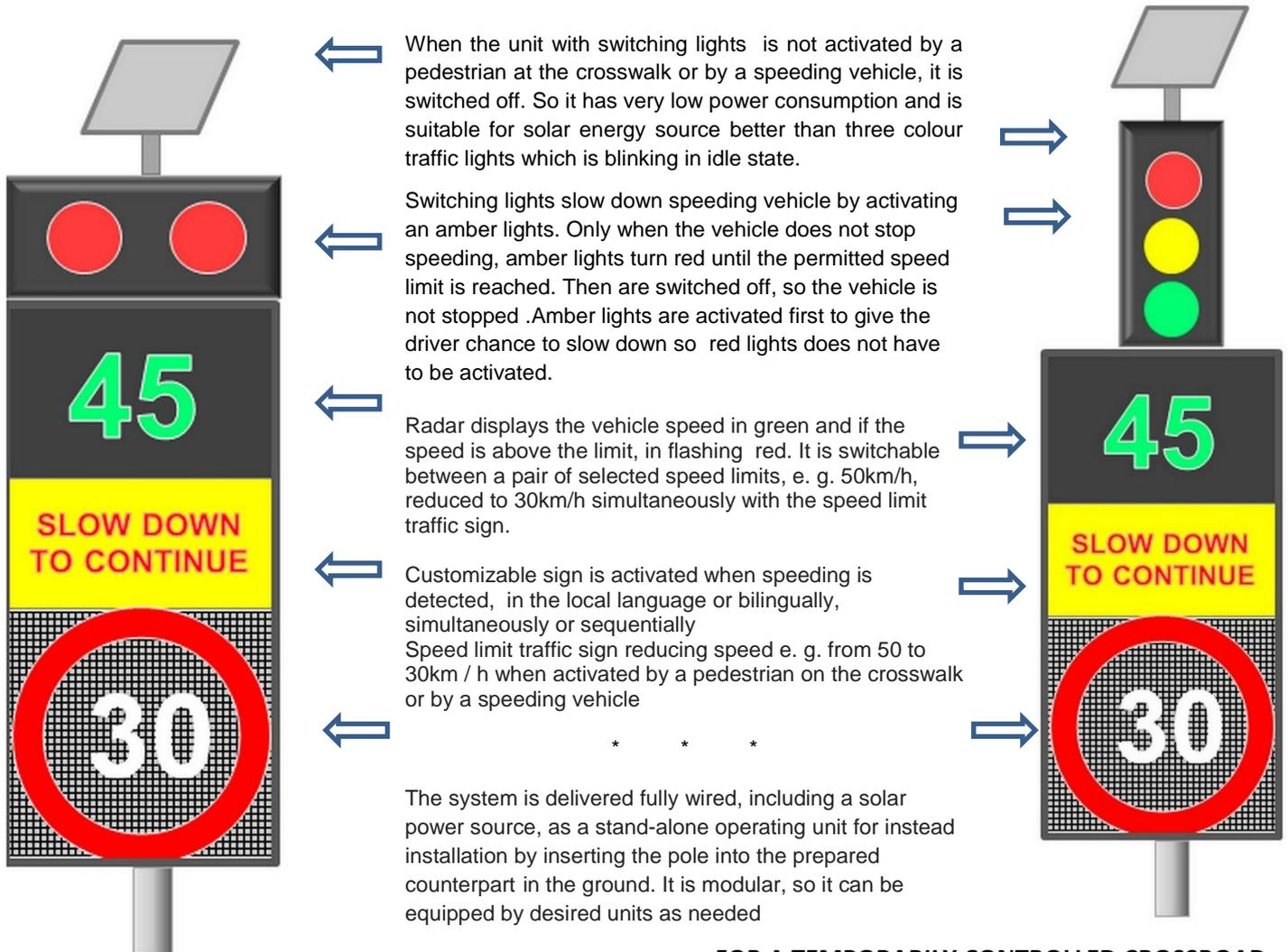
The intersection is normally uncontrolled so the traffic lights are turned off. Vehicles on the main road have priority. A pedestrian activates the compact crosswalk signalling and in the same time the speed limit sign 30 to slow down vehicles. It works as the uncontrolled crosswalk (see other side).
